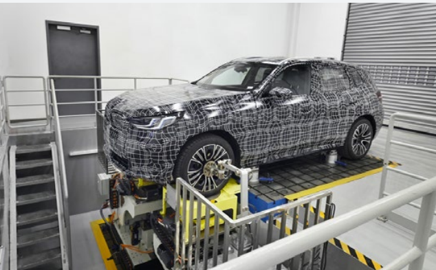
The chassis simulation kinematics and compliance lab.
