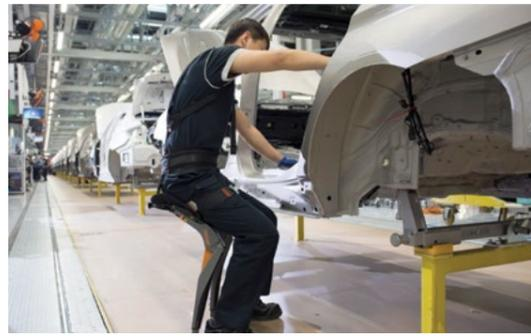
▶ A worker wearing an exoskeleton on the assembly line.
