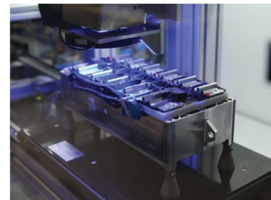
► 3D camera optical check of laser welding.
